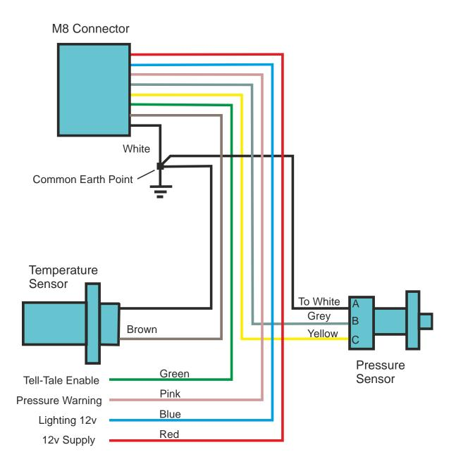
These are the connections for all gauges except fuel level gauges – see Section 6. If the gauge is a pressure gauge, then ignore the wires used for temperature gauges and vice versa. Of course, you must connect both temperature and pressure wires for dual pressure and temperature gauges.
