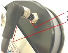
This pip should align with the cable direction
